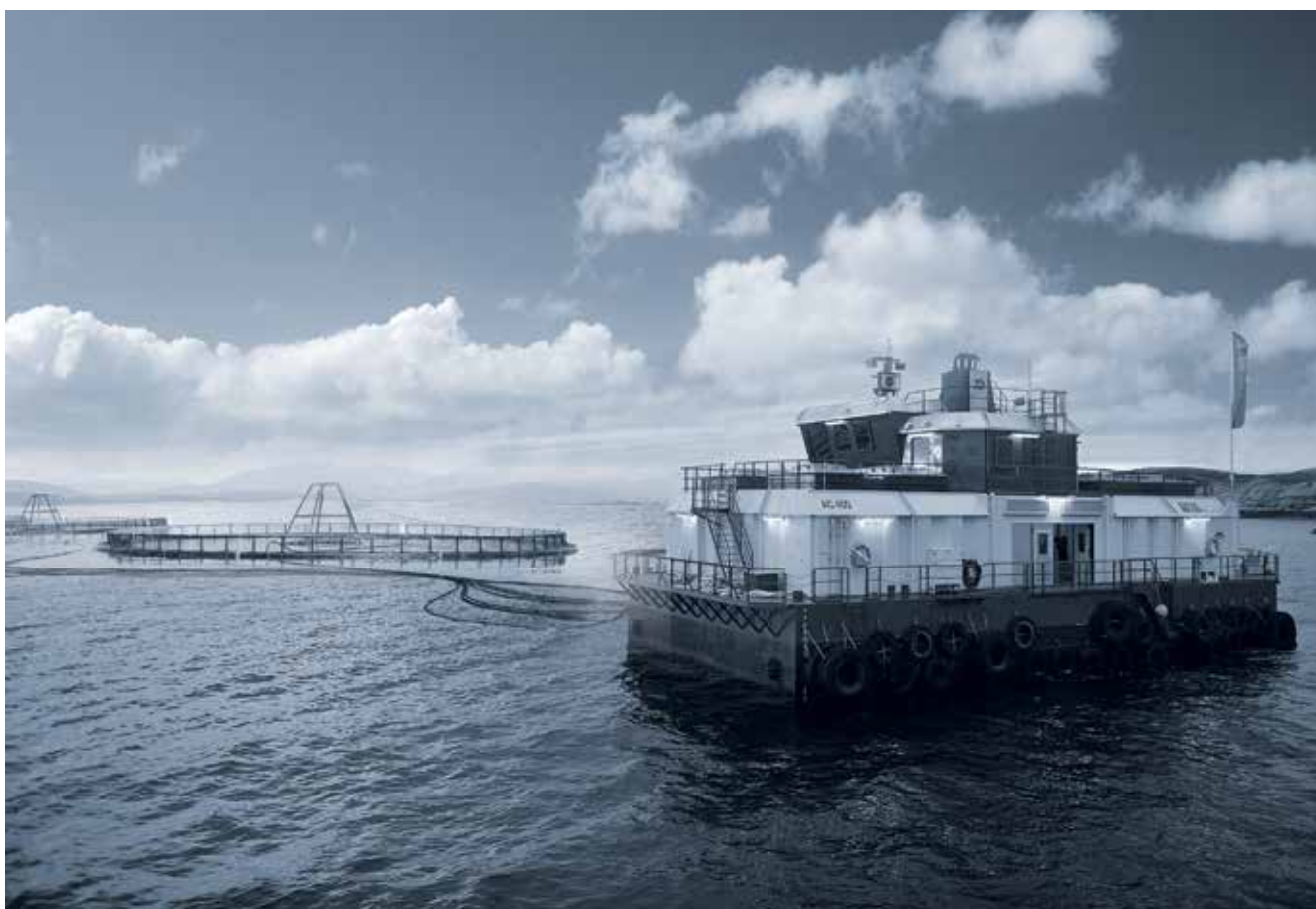
AKVA group's feed barges have load capacity from 96 to 850 metric tons.
