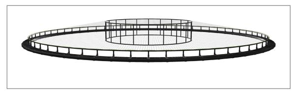
Bird net installed above hamster wheel, with the same mesh size as the whole skirt
