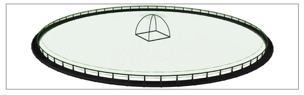
Bird net installed above centre floater, here shown with jump skirt
