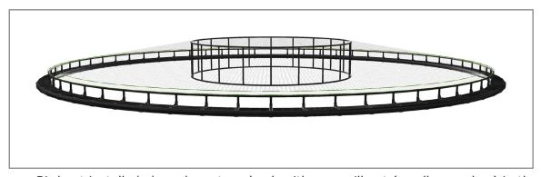
Bird net installed above hamster wheel, with overspill net (smaller meshes) in the lower part of the skirt – stops at handrail
