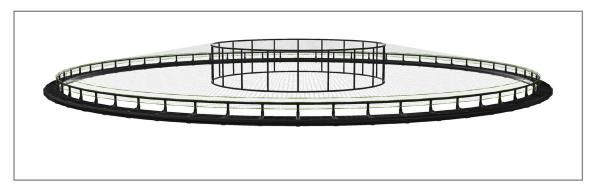
Bird net with overspill net in the lower part of the skirt, below the handrail. Can be made with a smaller meshes, or with the same mesh size as the skirt
