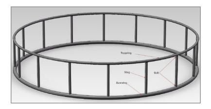
Hamster wheels are normally made from PE (polyethylene) and are available in various sizes. The height and diameter vary as required. It is important that there are no sharp edges, as the bird net may rest on the hamster wheel.
