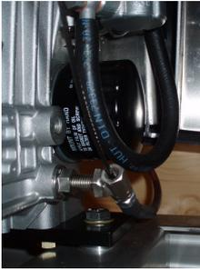
Use filter forceps to remove the motor's oil filter.
