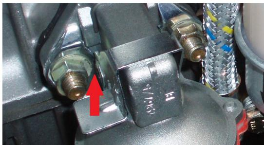
The ventilation handle is placed next to the diesel filter. Press the handle upwards several times, until a smooth resistance is felt.
