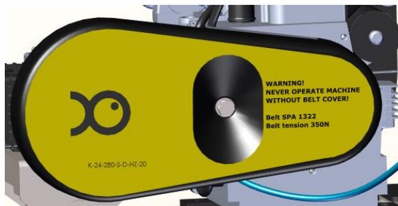
Remove the cover and check tightness by placing one hand on top of the belt and press down. The belt should be able to press about 2cm down.
