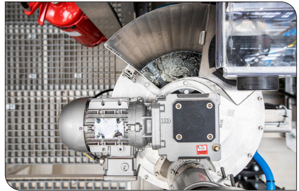
Illustration 5: Water sluice components
